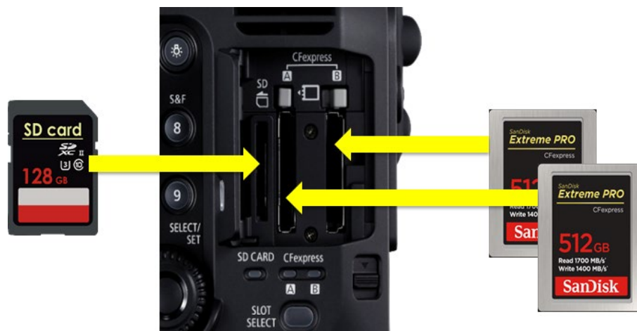
Figure 42 Two CFexpress 2.0 cards record the 5.9K Cinema RAW Light or the 4K XF-AVC file formats and an SD card records the Proxy video
