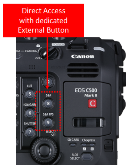
Figure 49 A new direct access to the Slow / Fast Motion mode offered by a dedicated button
