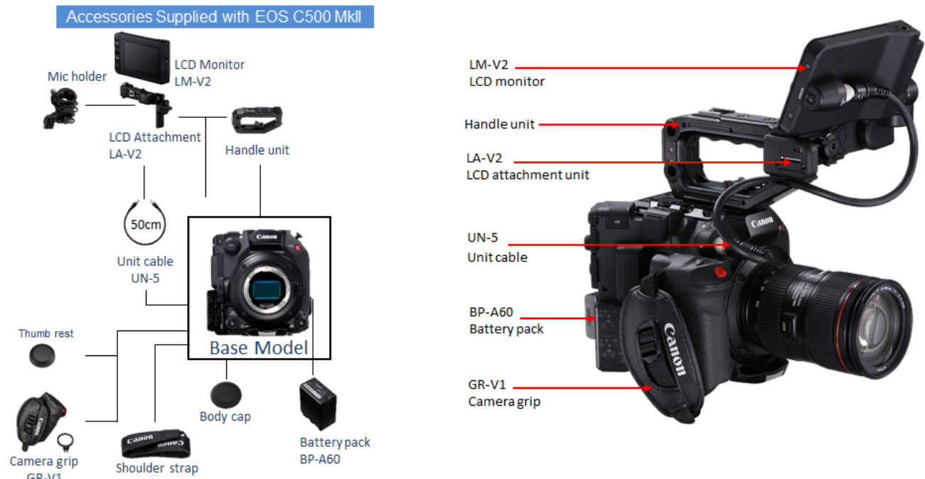
Figure 14 Showing the selection from the supplied accessories with the EOS C500 Mark II camera that configure a compact single operator acquisition system
