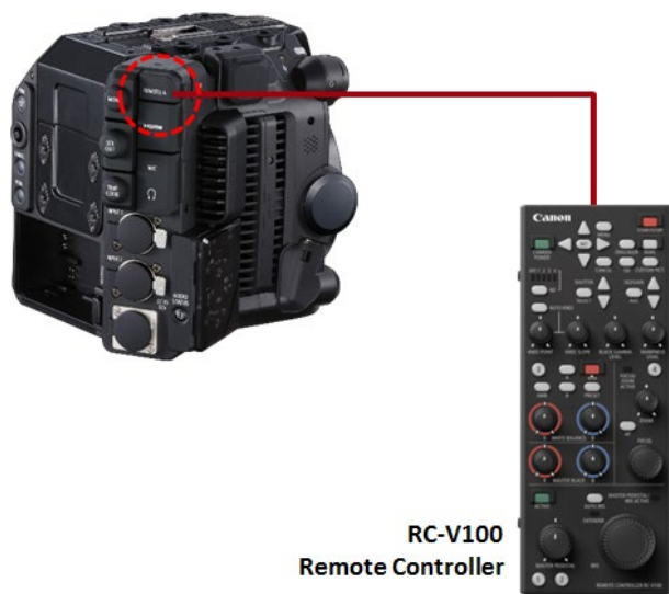
Figure 53 The RC-V100 video control panel supports remote control of video and also lens zoom, iris, and focus (including the Canon CINE SERVO lenses)
