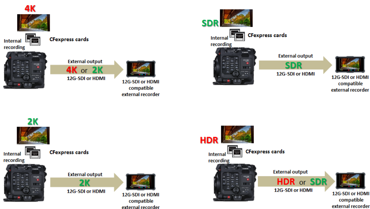
Figure 27 Allowable combinations of on-board and external recording of HDR / SDR and 4K / 2K
