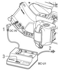
1 Connect the DC power output cable of the BC-U1/U2 to the DC IN connector of the camcorder.
