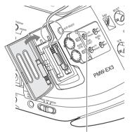
Pass through the cable guide slot.
